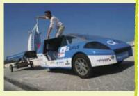
The car pulls a trailer loaded with six square meters of solar panels. The panels absorb sunlight and produce electricity. The power is then fed into a battery which drives the car. It took Palmer three years to build his car, with the assistance of scientists at four universities and financial help from 15 Swiss companies. The car can cover 100 km a day.
